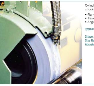
Cylindrical wheels are used most often when the part is held between centers and in chucks. There are three methods of cylindrical grinding: plunge, traverse, and angular.
