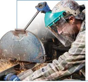
A chop saw is a light, low-horsepower portable machine. Although very similar to a compound miter saw, it is designed for cutting denser materials, like metal bar, tubing or pipe. Chop saw cut-off wheels are designed specifically for this machine with finer grit, softer grades, and reinforcement layers that match the application.
