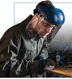
The Norton small diameter cut-off wheel line consists of Type 01/41 straight and Type 27/42 depressed center cut-off wheels from 1-1/2" to 9" diameters. These wheels come in ultra thin .035" for quick burn-free and burr-free cutting to .125" for more durable applications. All are reinforced for the demanding nature of portable cut-off.
