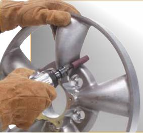
Cartridge rolls are strips of abrasive cloth rolled and glued to form a solid shape that is designed to break down during use and reveal the next layer of abrasive. A valuable abrasive tool for reaching into corners, where larger diameter tools cannot work
